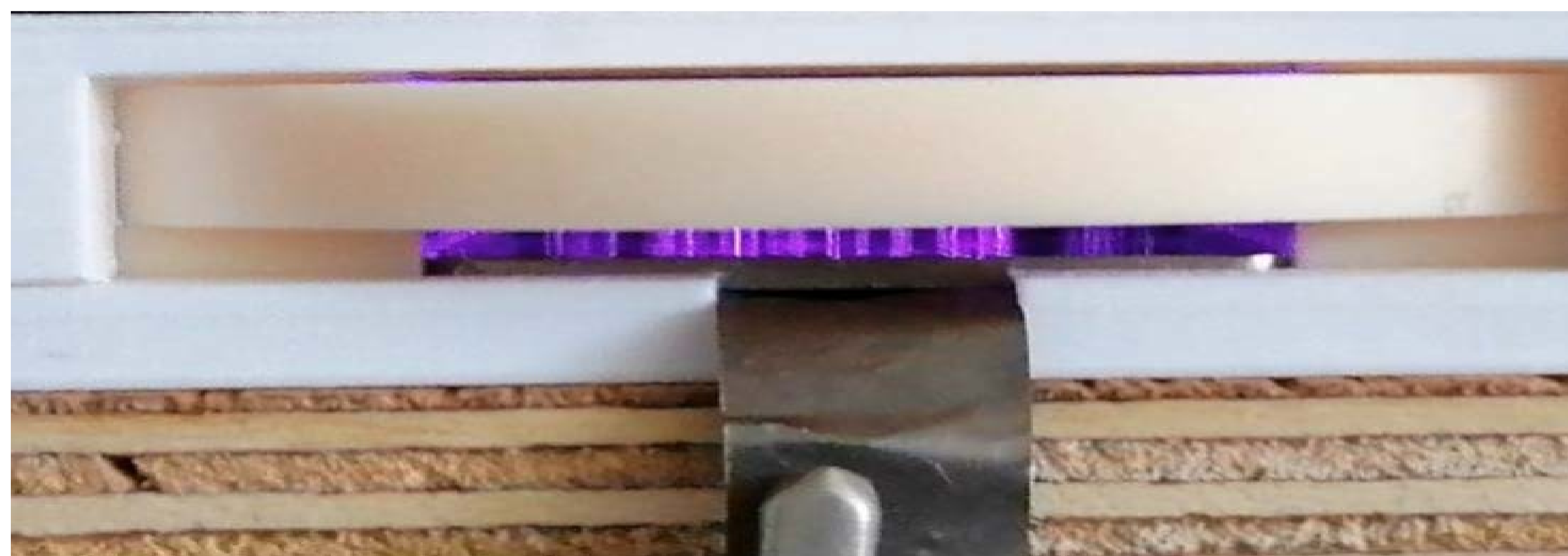
Fig. 1 : In-house atmospheric DBD-plasma reactor for the treatment of polymer foils
